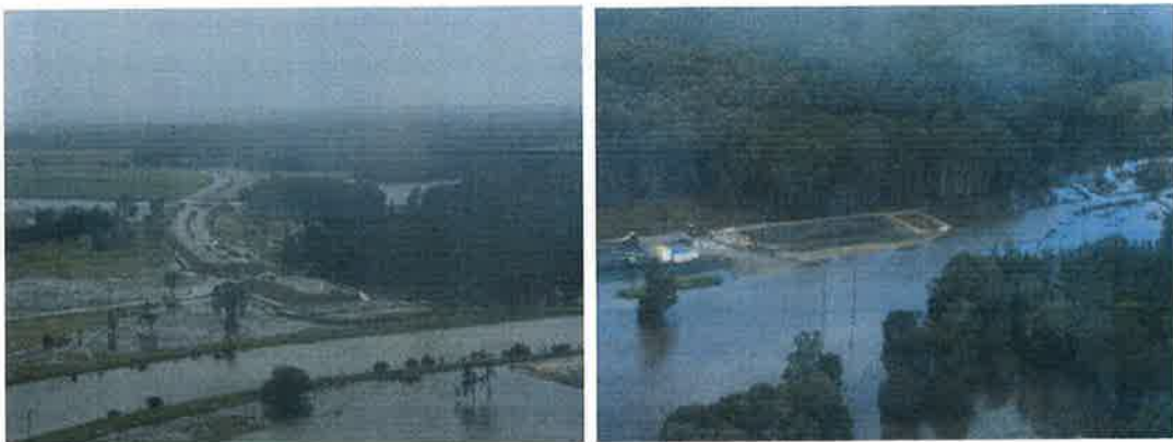
Fig 8. Water banked on the western side of the carriage way embankment, north and south of the Canal, after heavy rain in 2017
